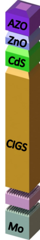
Fig. 4. Modified model with the synthetic dielectric spacer layer. Thicknesses of different layers (in nm) from top to bottom are as follows: 250, 60, 70, 1600, d and 320. The thickness d of the spacer layer was varied between 20 nm and 170 nm.
