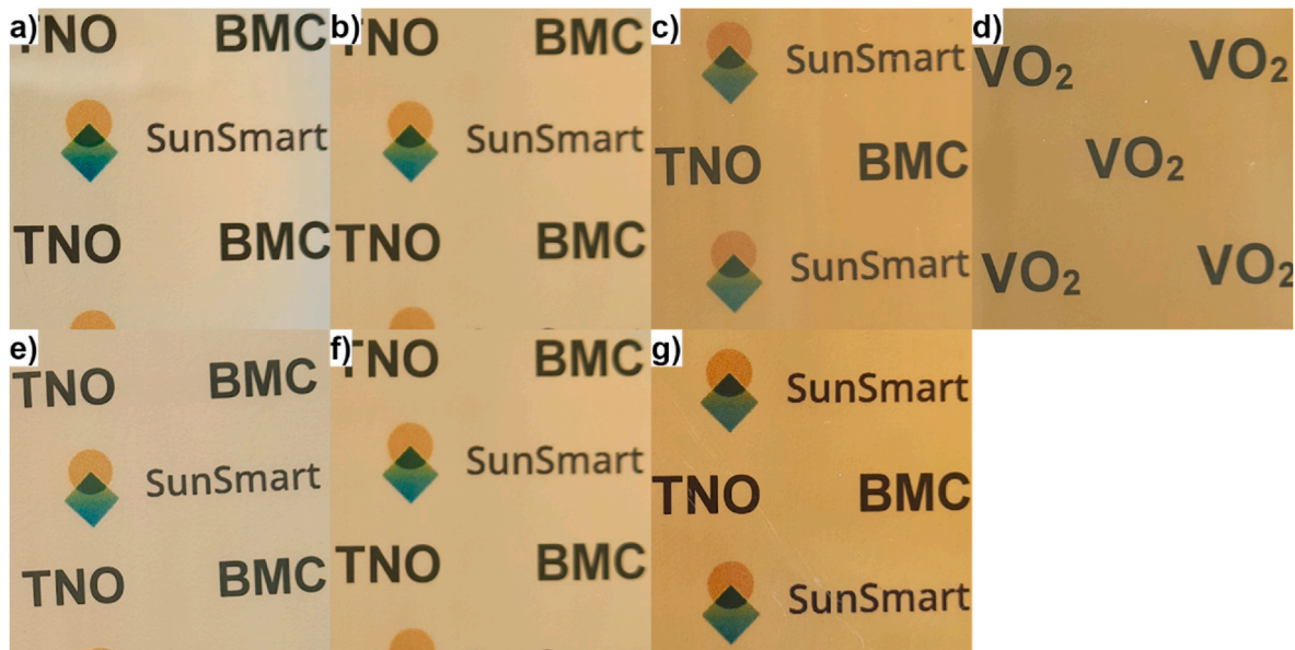
Fig. 3. Thermochromic coatings at layer thickness around 100 nm and varying composition of a) 40% v/v (1), b) 50% v/v (2b), c) 70% v/v (3), d) 100% v/v \text{VO}_2 , and coatings at 50% v/v \text{VO}_2 at varying layer thickness of e) 47 nm (2a), f) 96 nm (2b), and g) 140 nm (2c).
